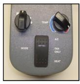
This may in some cases cause the engine to overheat. In the MAX temp setting, the valve sends ALL the water to the under-bunk module. The fan needs to be on high to dissipate the heat, since the under-bunk is now performing as a radiator.
